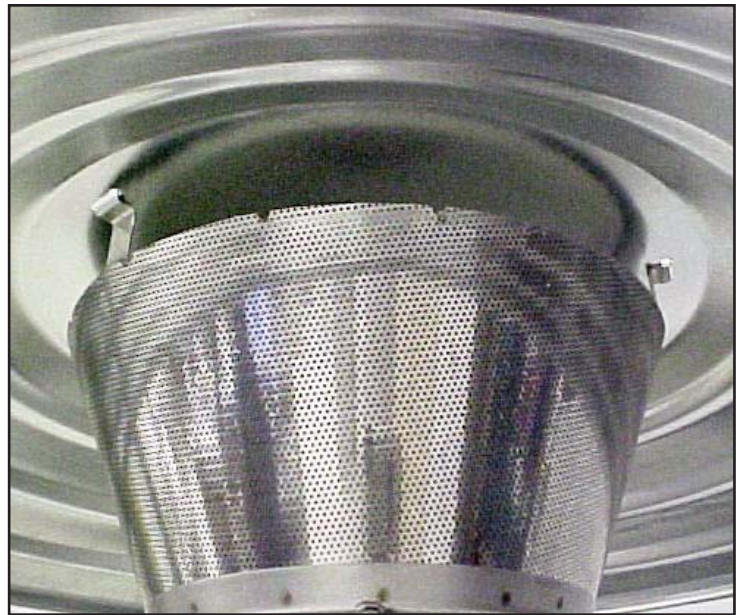
(1) Place CONE INSULATION inside the EMITTER .
